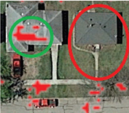
Identify determines green circled home on the left has coverage for desired install height above roof and red circle home on the right does not. Location and addressing information is provided for the home on the left and all similar buildings.
