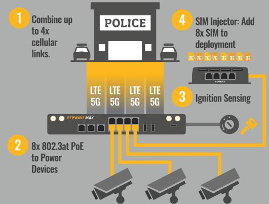
The HD4 MBX combines the bandwidth of 4x Gigabit LTE links into a fast, reliable, and secure SD-WAN connection, enabling you to stream high-definition video in real-time. This can all be achieved without investing in any infrastructure. With SpeedFusion-enabled devices on multiple vehicles and aerial resources, you can monitor the situation from multiple perspectives without needing a line-of-sight connection.
